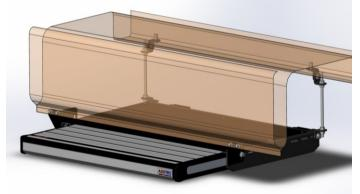
Define the place for the 4 mounting bolts on the front. The holes for this fixation should be drilled in the lower flange of the outer chassis bar of the vehicle. Drill the holes Ø6.5 mm. Always protect all drilled holes with zinc spray. Make sure there is enough material in the flange under the hole. Place the step with two bolts at the flange and support it at the rear.
